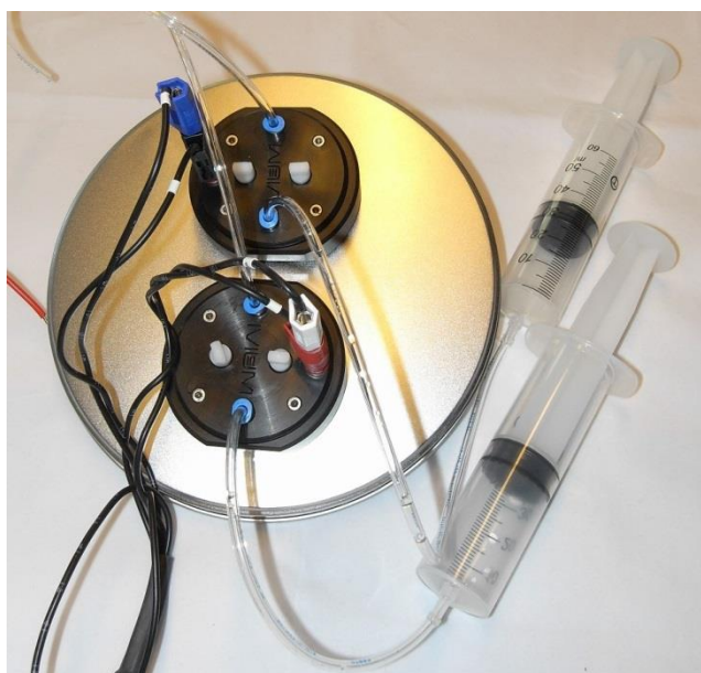
Figure 3: Connection of two MCF cells in a 2-electrode configuration
