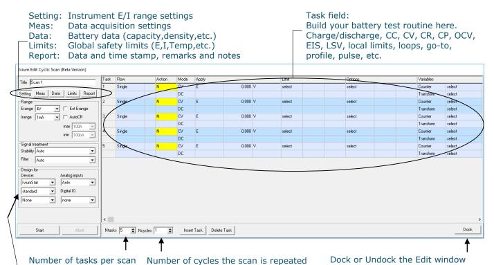
Design a scan for this instrument; checks settings against instrument capability when instrument is not connected.
