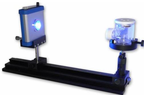
Optionally included with the Optical platform is a water jacketed 40ml glass cell that fits the cell positioning clamp. The glass cell is equipped with a quartz glass window to allow the light to pass through. A lid with a sealing ring is provided with 3 openings for the counter electrode, reference electrode and working electrode.
